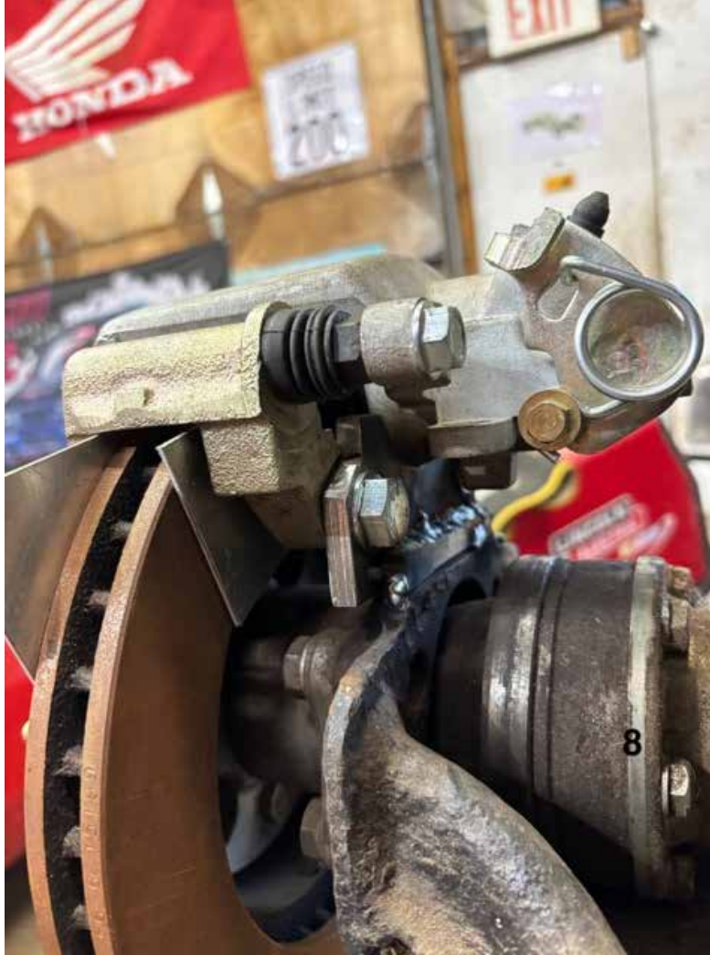
Picture 8 shows the caliper in place with the aluminum shims and the mount tack welded to the control arm.
