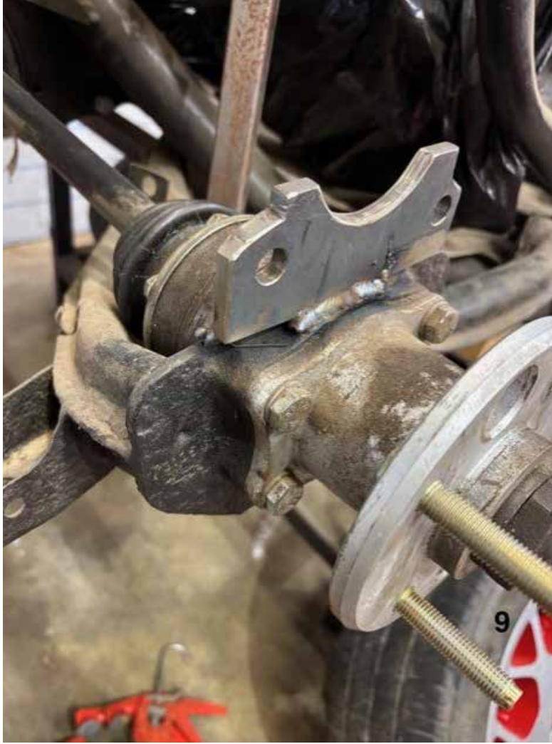
Picture 9 shows the finished outer weld. You can see how close it is to the bearing mount
